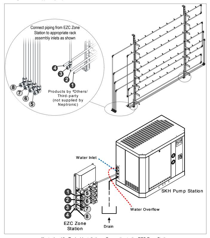
Illustration 13 - Typical Installation – Connecting to the EZC Zone Station
