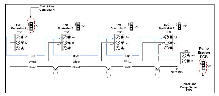
Illustration 25 - Pump Station to EZC EOL Setup
