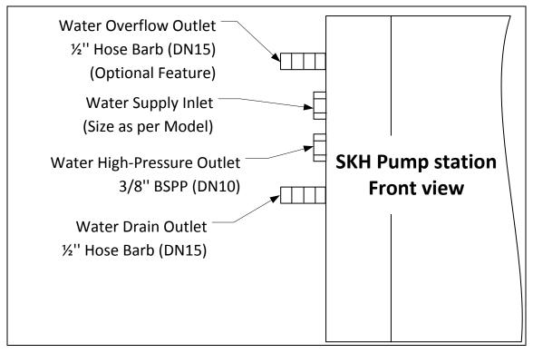
Illustration 15 - Water Connections - Pump Station
