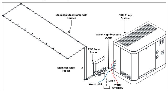
Illustration 7 - Typical Installation with Rigid Nozzle Ramp
