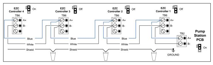
Illustration 23 - Pump Station to EZC Control Connections (Multiple EZCs)
