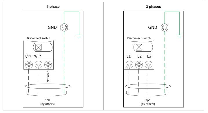
Illustration 17 - Power Supply Connections on SKH Pump Station
