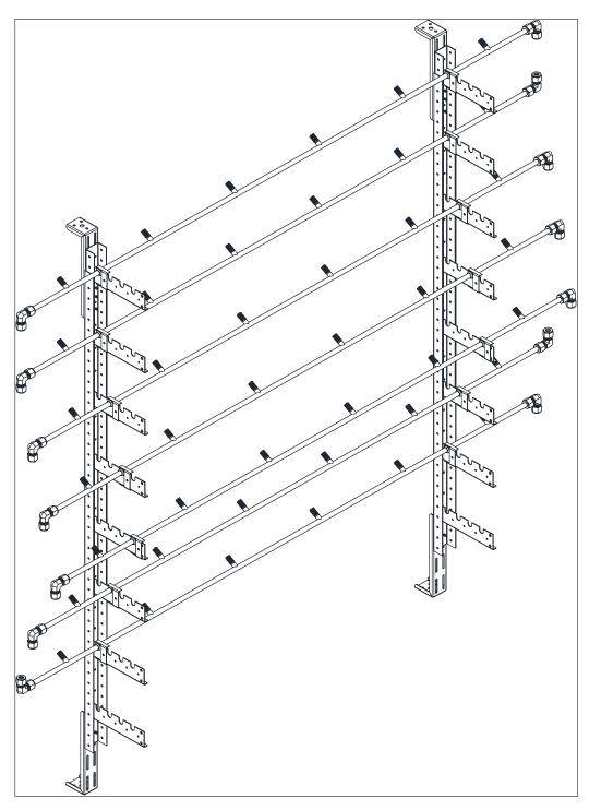
Illustration 12 - Rack Assembly within a Duct
