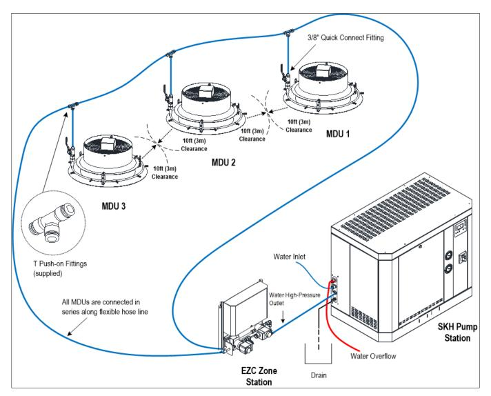
Illustration 10 - Typical Installation of MDU to EZC
