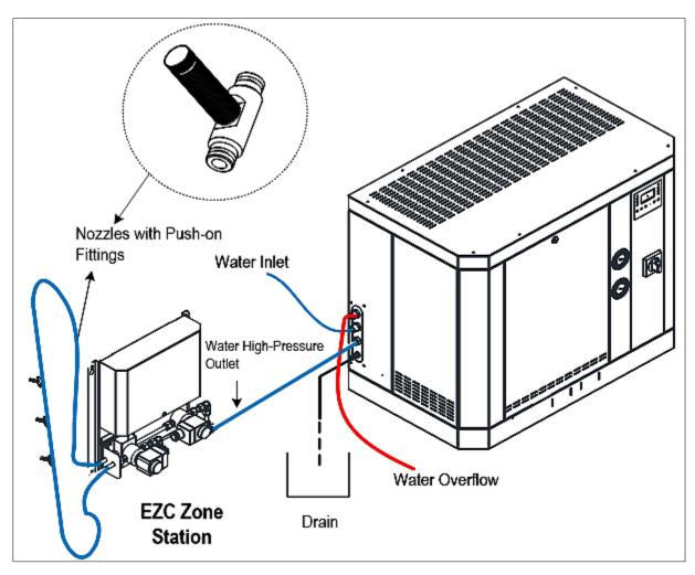
Illustration 8 - Typical Installation with Flexible Hose
