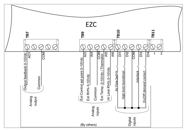
Illustration 19 - SKH Controller Wiring Diagram
