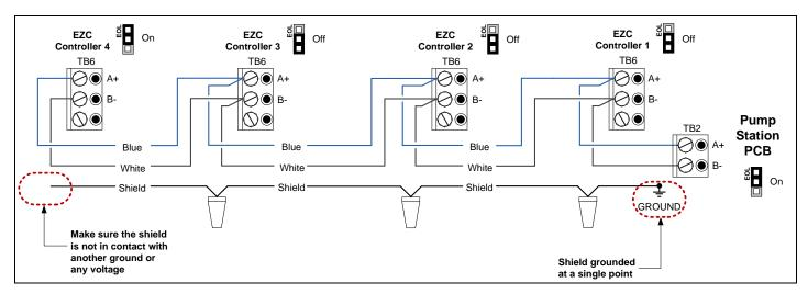
Illustration 24 - Pump Station to EZC Shield Wiring
